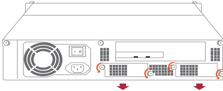
2. The rear 75×75×28 mm blower fan speed can be adjusted. As the blower fan module is pulled out, there are four sets of jumpers labeled with 6V, 8V, 10V, 12V from top to bottom on the fan connector board. The default setting is the jumper being placed over pin 7 and 8 for label 6V for slowest speed. The speed increases from label 8V to label 12V. As jumper is not placed over pins, the fan will spin at 12V full speed.
