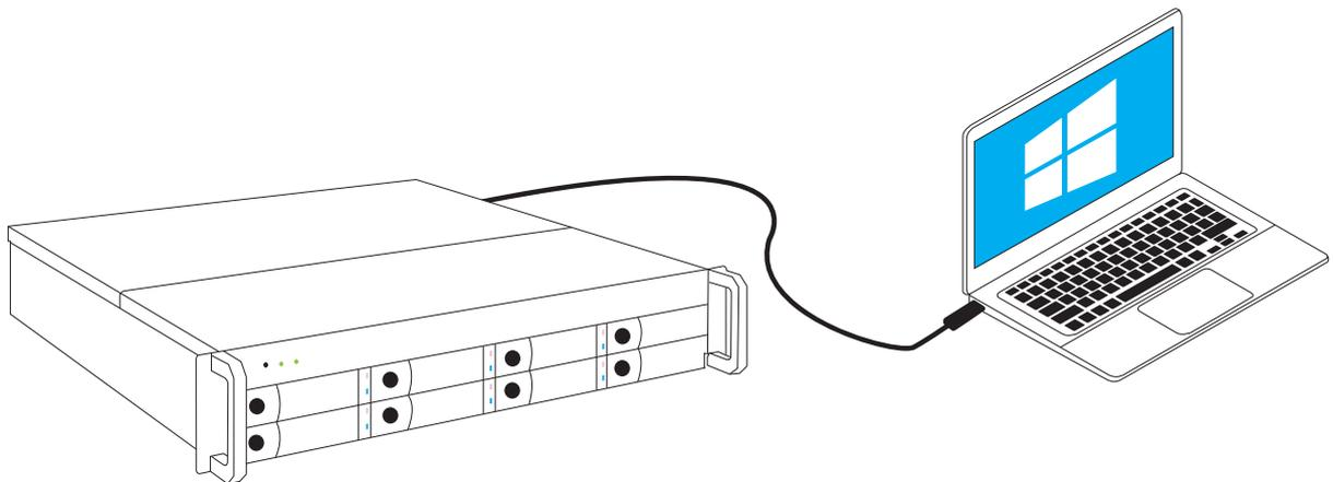
2. As NA341TB3 storage is connected to computer by Thunderbolt cable, when shutting down computer, the NA341TB3 will be shut down automatically as well.
