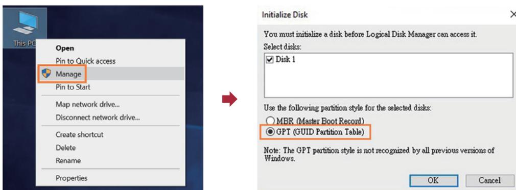
9. Following selecting GPT (GUID Partition Table), the RAID volume will appear in the center field of the window. Right click the section of the RAID volume, and select **New Simple Volume** to format the RAID volume.
