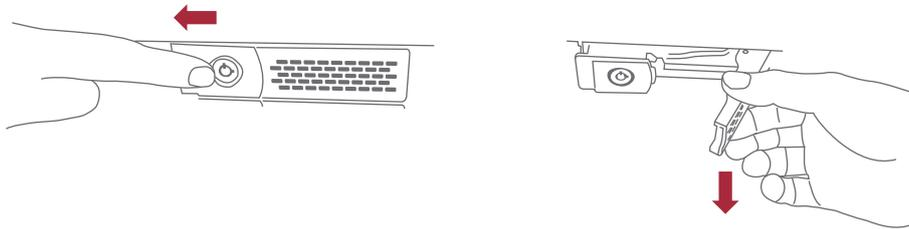
3. Place HDDs in the trays and fix them with the included hard drive mounting screws. And then put the trays with HDDs back to NA341TB3 storage.
