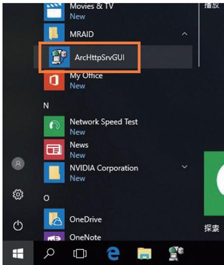
5. Subsequent to running ArcHttpSrvGUI application, the web-based GUI will appear. Select **SAS RAID Controllers**, and then select **Web Management** to enter the web GUI
