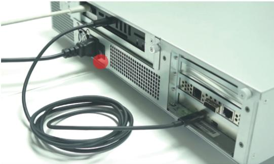
2. As the embedded Mac mini is connected to Netstor unit by Thunderbolt 3 cable, press and hold the LED power button in front of NA338TB3 for three seconds until the LED button shows blue light. The built-in solenoid actuator at rear of enclosure will push Mac mini's power button to have Mac mini and whole system be powered on.
