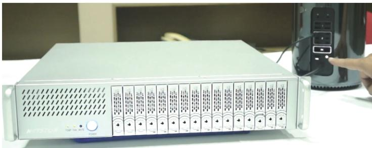
3. As computer is connected to NA338TB3 unit externally by Thunderbolt 3 cable, while shutting down the host computer through operating system, the NA338TB3 unit will be powered off simultaneously as well.
