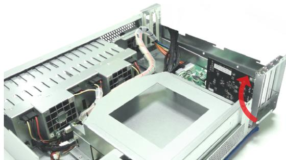
4. Three PCIe slots at rear of PCIe expansion unit are covered by removable L-shape metal brackets. After unscrewing the screw of the L-shape metal bracket, the PCIe slot is ready for the third-party PCIe card installation.
